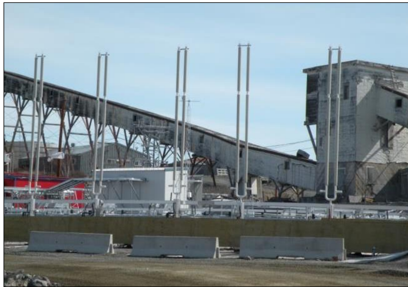
Thermosyphon test plot, Giant Mine (author photo)
